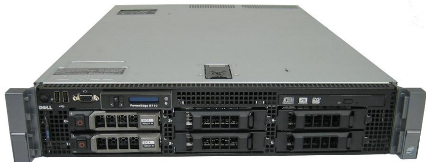
Figura N° 24: Servidor Dell PowerEdge R710– 3.5” Model
