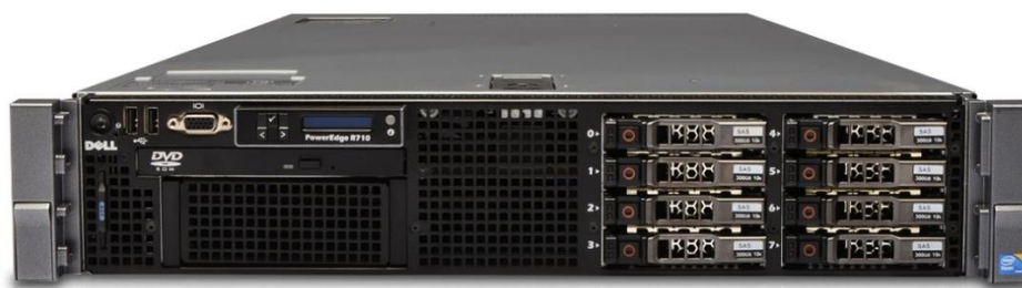
Figura N° 16: Servidor Dell PowerEdge R710 -2.5” Model.
