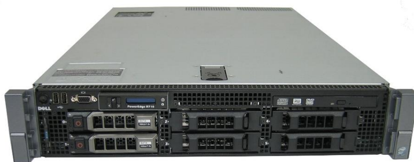
Figura N° 15: Servidor Dell PowerEdge R710 - 3.5” Model.
