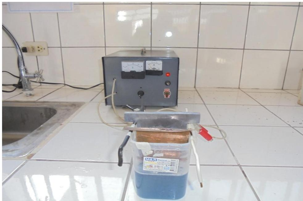
**A.6.-VISTA DE ANODO (PLOMO) Y CATODO (COBRE)**
