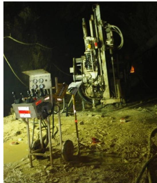
Figura 1 Perforadora de taladros largos Stoper Master
