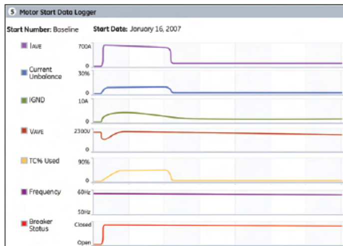
Troubleshoot faults that occur during motor starts using the Motor Start Data logger.
